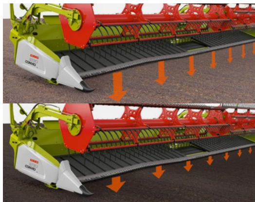
ACTIVE FLOAT allows ground pressure to be adjusted from the cab
