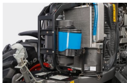
The engine air filter is in front of the radiator and easy to reach from the ground.
