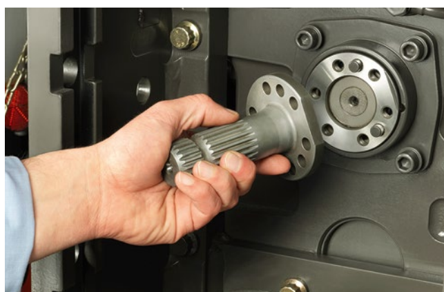
The PTO stub can be changed easily.
