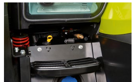
Compressed air connection on the left side of the access steps.
