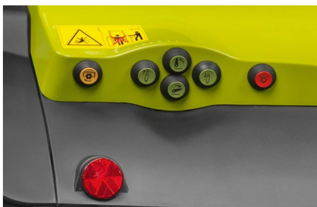
External controls for rear PTO.
