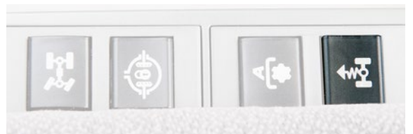
Switch to activate front axle suspension.
